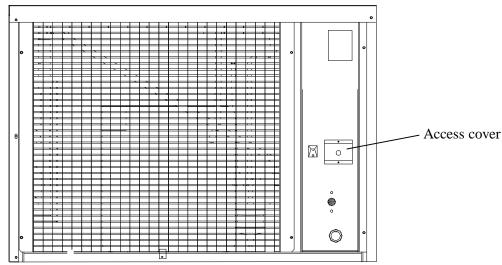
1. Unscrew the two screws holding the access cover and remove the cover. You will find two leads (black and white). See drawing below.
